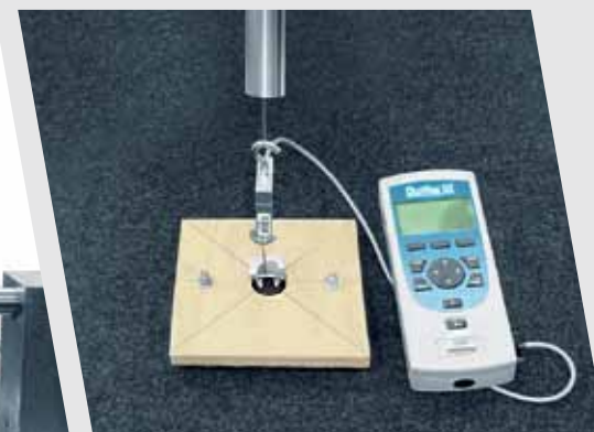
Testing of fixing element strength
