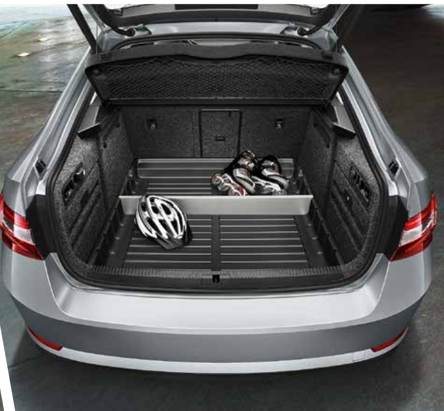
Plastic boot dish can be additionally equipped with Aluminium partition (3T0 017 254)
