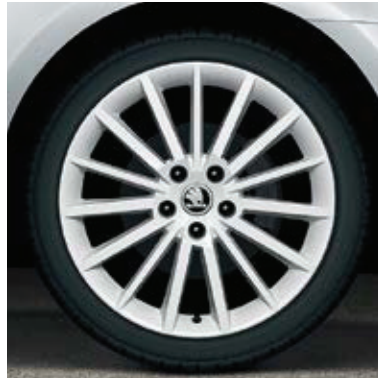
Alloy wheel 7.5J x 18" Turini for tyre 225/40 R18 in white design (5E0071498AFM9)
